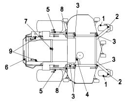
c) Lubricate front caster pivots once a year. Remove hex plug and cap. Thread grease zerk in hole and pump with grease until it oozes out around top bearing. Remove grease zerk and thread plug back in. Place cap back on.
